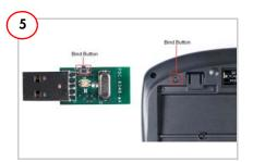
Press the bind button on the bridge; the red LED blinks. Press the bind button on the keyboard to bind it with the bridge. The mouse and keyboard work smoothly with the PC.
